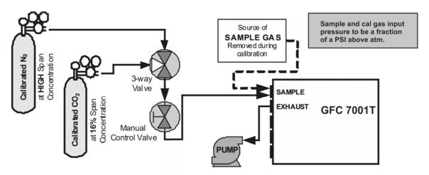
Figure 9-8: CO<sub>2</sub> Sensor Calibration Set Up
